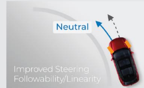
Electric Power Steering-Variable Gear Ratio (VGR) Electric power steering with variable gear ratio
